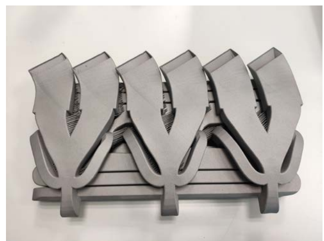
Figure 5: PJA actuator manufactured by SLM and post-processed.
